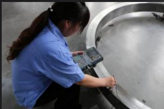
U.T. test of forging material
